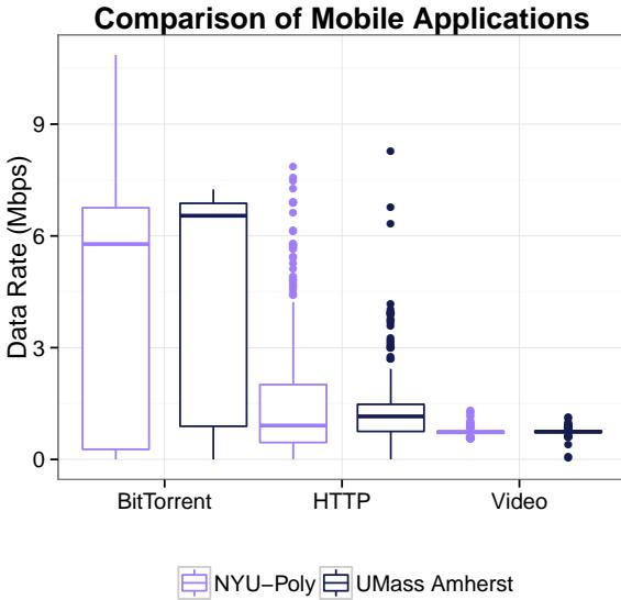
**Fig. 8:** Measurements from mobile experiments. The boxplot shows the mean data rate for each experiment, with the upper and lower hinges corresponding to the first and third quartiles. Outliers beyond 1.5 interquartile range (IQR) of the hinges are plotted as points.
