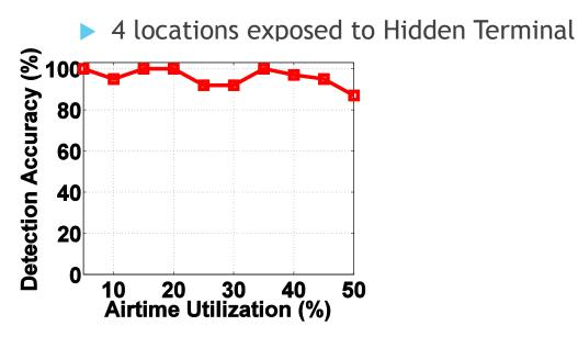
Detection Accuracy > 85% for varying Airtime Utilization of Hidden Link
