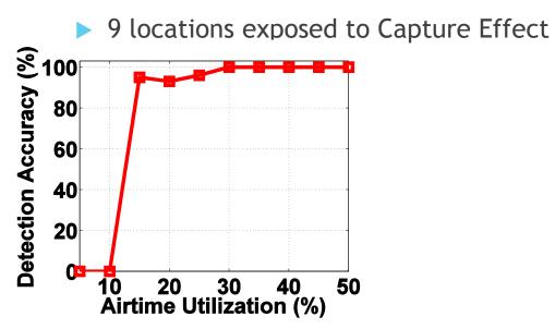
Low Airtime Utilization leads to similar impact as of Hidden Terminal -Failure in detection
