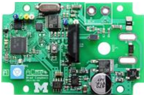
AC Energy Monitoring
