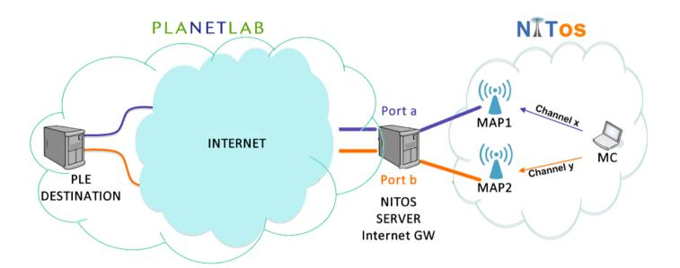
The experimental scenario is implemented in the federated NITOS - Planetlab Europe testbeds
