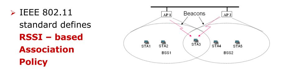
A STA simply selects the AP from which it has received the strongest signal during the scanning process.
