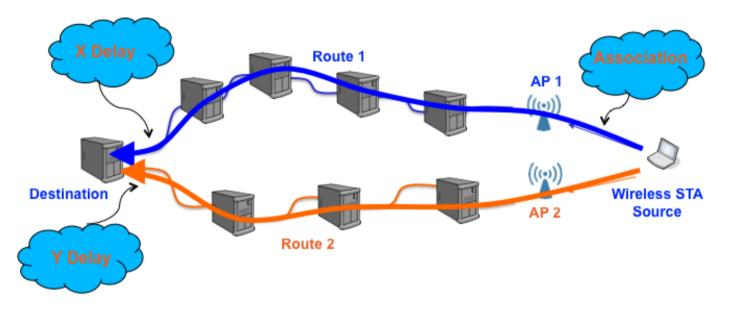
The wireless STA decides about its association based on the end-to-end delay on both the wired and the wireless part.
