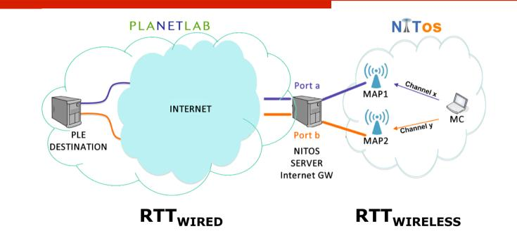
**RTT<sub>WIRED</sub>** : estimated through probe packets that are transmitted from the APs and are destined to the PLE node
