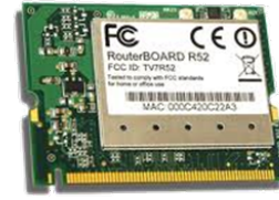
Fig. 3: The Mikrotik R52 Card for 5.9 GHz band operation
