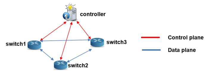
• Every time a new packet arrives to the router and there is no entry in the flow table for it, the router communicates with the controller.
