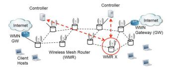
Fig. 3. Controller selection by a Wireless Mesh Router
