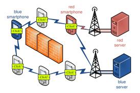
(a) An enhanced wireless access network with cooperative diversity. EBoW [15] uses efficiently both paths for the forwarding of the traffic generated by the blue smartphone and forwarded to the blue server.
