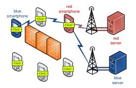
(b) SRCR [14] uses only the shortest path to forward the traffic generated by the blue smartphone, which passes through the overloaded red smartphone.
