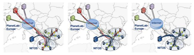
(c) Server Request mapping for the Client-based (d) Server Request mapping for the Load-based (e) Server Request mapping for the Proximitypolicy based policy
