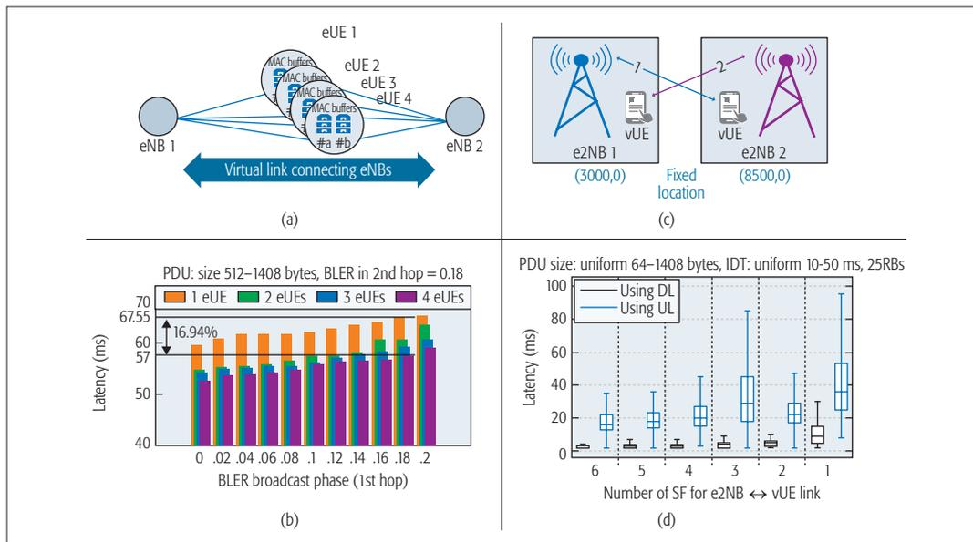
**Figure 4.** Logical topology for the performance evaluation scenario in OAI: a) four eUEs are leveraged to interconnect two eNBs; b) performance results for latency in the eUEs scenario; c) two e2NBs establish link connectivity using vUEs; d) performance results for latency in e2NB-vUEs scenario.
