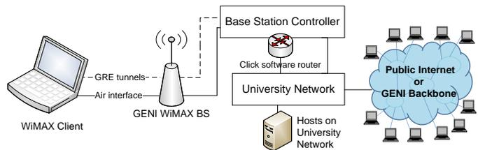
Fig. 1: The WiMAX testbed network configuration. A software router configured by the BS controller forwards traffic from each client to its predefined datapath on the university network, the public Internet, or a GENI backbone link.
