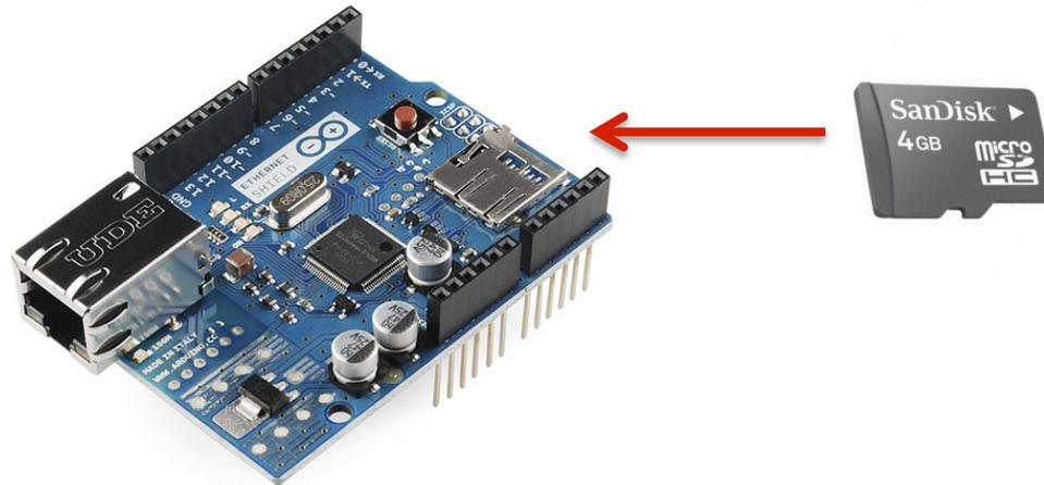
**Ethernet Shield with attached SD card**
