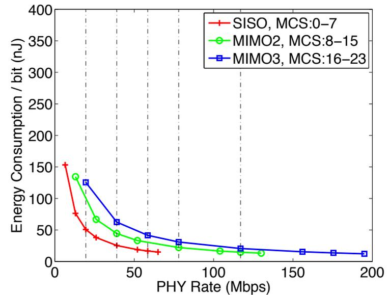
Proper Activation of the required number of RF-chains can increase energy savings up to 60%
