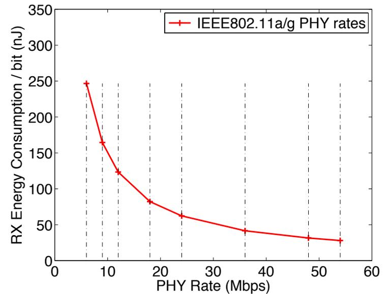
Increase of PHY bit-rate efficiently reduces Energy consumption/bit
