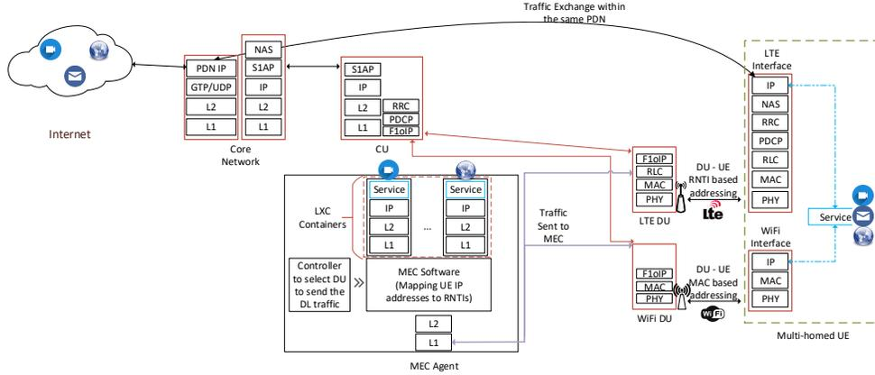
Fig. 2: Overall system architecture: F1oIP orchestrates the intercommunication between the CU and DUs, whereas the MEC software is providing the functionality of mapping RNTI to IPs
