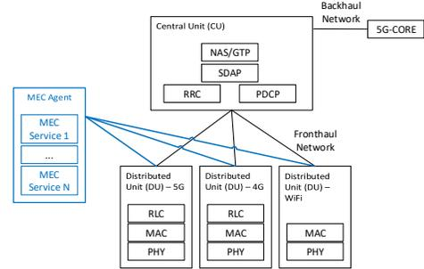
Fig. 1: Proposed base station architecture with MEC services being placed on the fronthaul interface
