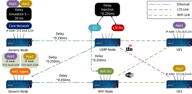
Fig. 3: Experimental topology for the evaluation of the MEC scheme in the NITOS testbed
