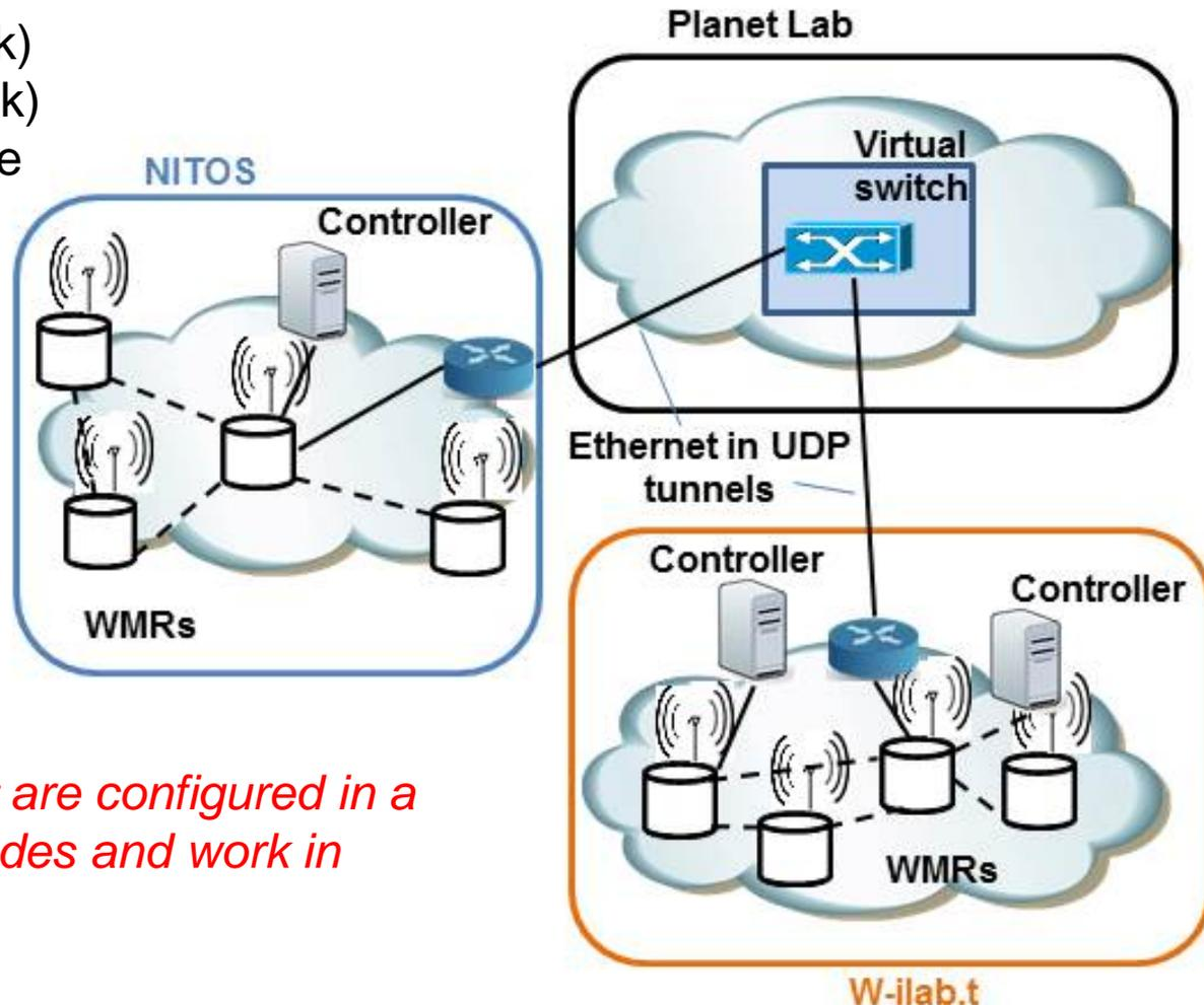
*Nodes from NITOS and w.llab.t are configured in a way to act as wireless mesh nodes and work in parallel as OpenFlow switches*
