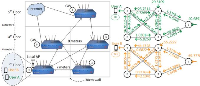
Fig. 2: Wireless Mesh Experimentation Topology: (left) NITOS interior building testbed setup. (right) Optimal flows for mobile users A and B (Kbits).
