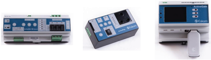
Figure 7.17 Active devices (ActiveDIN on the left , ActivePlug center and ActiveGate on the right ).
