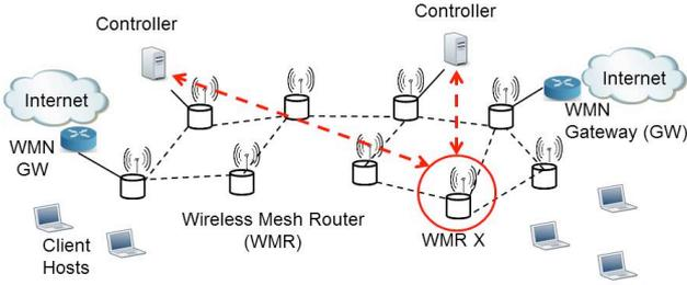
Fig. 3. Controller selection by a Wireless Mesh Router
