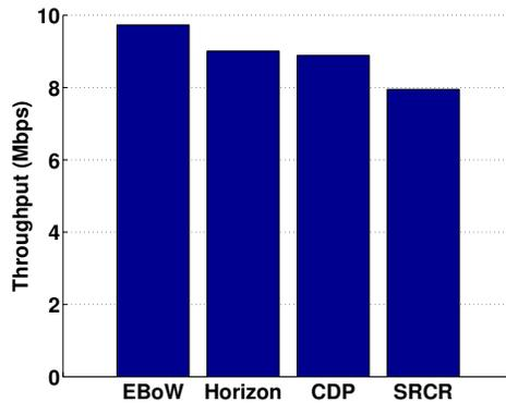
(c) Throughput performance of the four under investigation routing algorithms.
