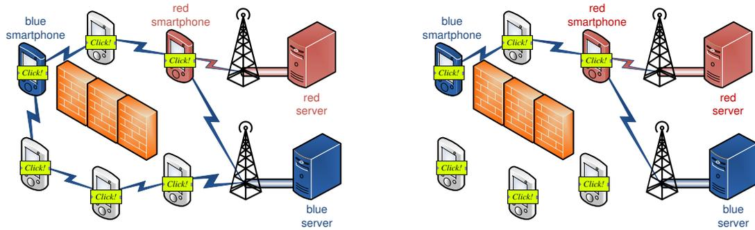
(a) An enhanced wireless access network with cooperative diversity. EBoW [15] uses efficiently both paths for the forwarding of the traffic generated by the blue smartphone and forwarded to the blue server.
