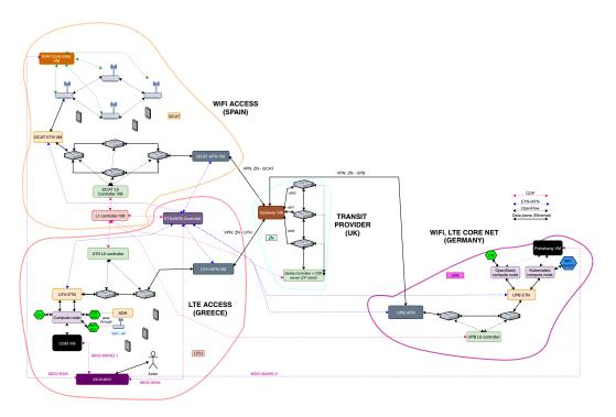
Fig. 3. Testbed set up to test multi-domain e2e RAN service provisioning
