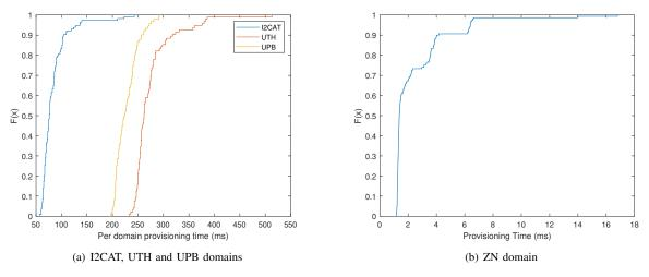
Fig. 7. e2e connection provisioning time broken per domain
