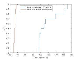
Fig. 8. Overall provisioning time for the virtual LTE and virtual Wi-Fi services
