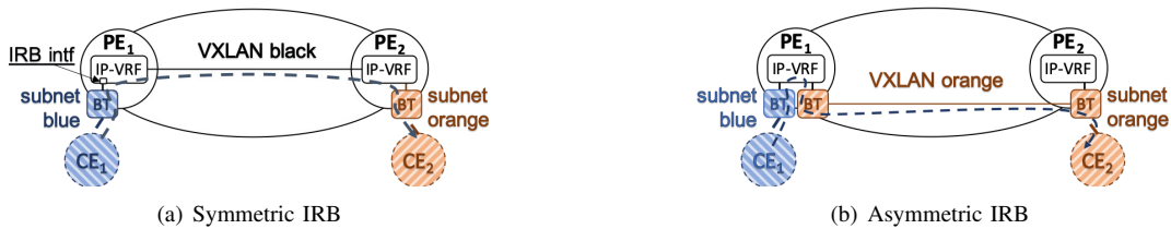
Fig. 2: IRB solution types for VXLAN based EVPN
