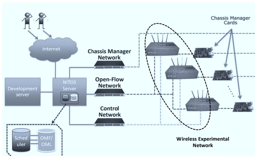
**Fig. 2.** Blueprint of the NITOS testbed architecture. NITOS testbed’s Control, Open-Flow, Chassis Manager, and Wireless Experimental Networks are accessed by remote users via the NITOS server. OMF and NITOS scheduler are software components residing on the NITOS server.
