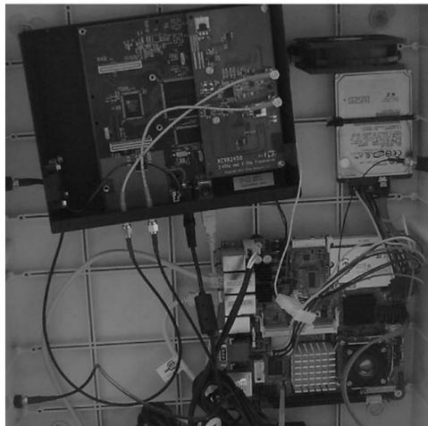
**Fig. 5.** USRP board mounted on NITOS node
