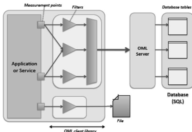
**Fig. 8.** Overview of OML architecture (source: <http://mytestbed.net>)
