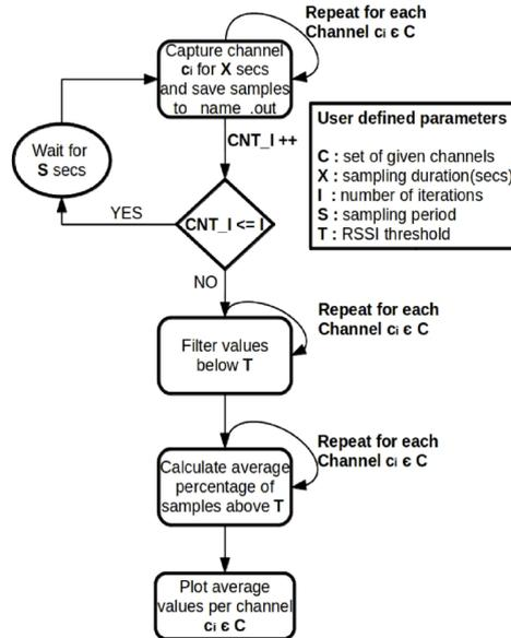
**Fig. 6.** Flowchart of the Channel Sensing Framework Procedure.
