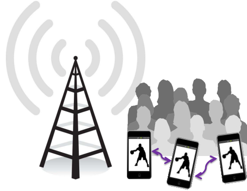
Figure 1: The principal network, which is an infrastructure-based cellular network, provides downlink multicast or broadcast services. The assistant network is an ad hoc cooperative network formed by physically co-located peers who are consuming the same media content, and is used to recover packets in a peer to peer fashion.
